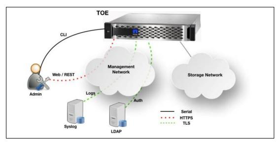
Figure 1: TOE Architecture
